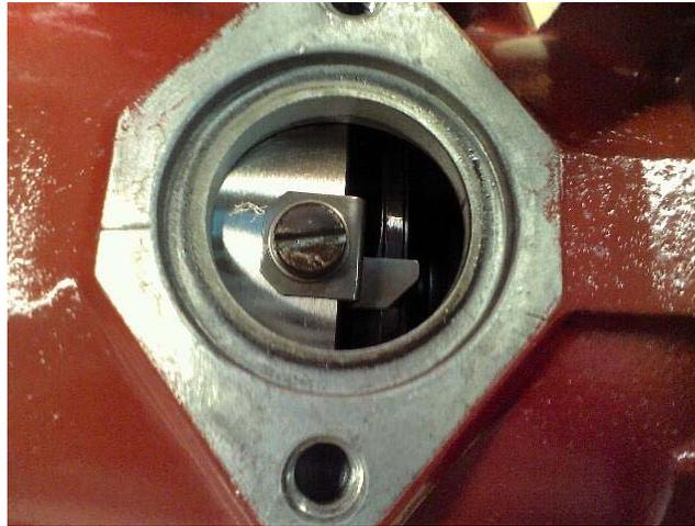
This line is can be faint and may be hard to see. If there is no line visible rotate the engine one complete revolution. Stop the engine rotation as the mark reaches the pointer and observe the timing pointer to the front pulley, as outlined in Picture 1. If it is on the correct degree mark for your engine, then the engine is correctly timed.
