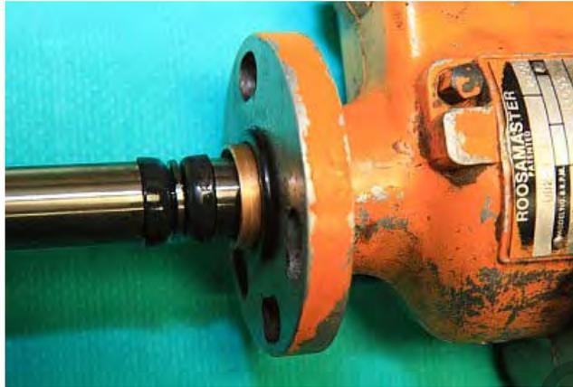
5. While compressing the drive shaft seal slide the pump into position over the driveshaft. Be very careful to guide the seal into place, if you roll the edge of the seal during installation you will have a major engine oil dilution problem. Install the pump as straight as possible to prevent the shaft from scoring the pilot busing in the injection pump.
