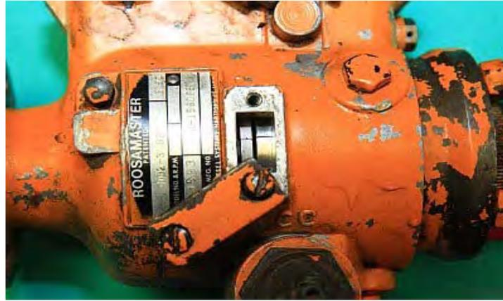
Timing marks on a DB model pump (figure 2)
